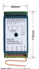
The **ET-RX3-RC** Universal Radio Receiver allows for Pulse, Latch or unique programmable up to 55 secs sustained/delay pulse output.
